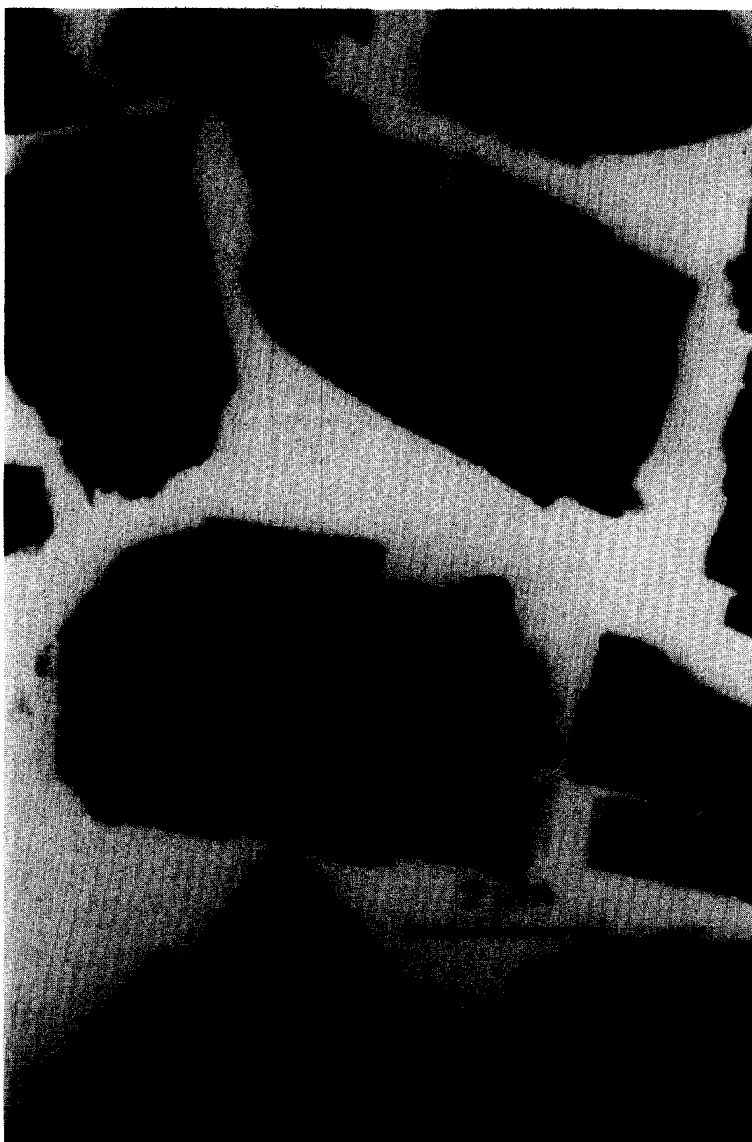
FIG. 1b. TE micrograph on the same sample as Fig. 1a, showing the microcracks.
